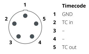
LTC Out Impedance  $1k\Omega$ LTC In Impedance 15kΩ
