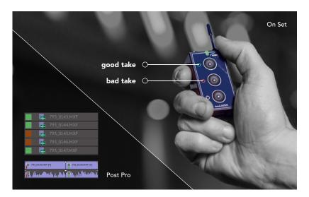
You can use your NanoLockit both as a Timecode Generator AND a Live Logger. The goal of the Logging feature is to mark good and bad clips (or several parts of a clip) directly on set. This can save loads of time in post-production.
